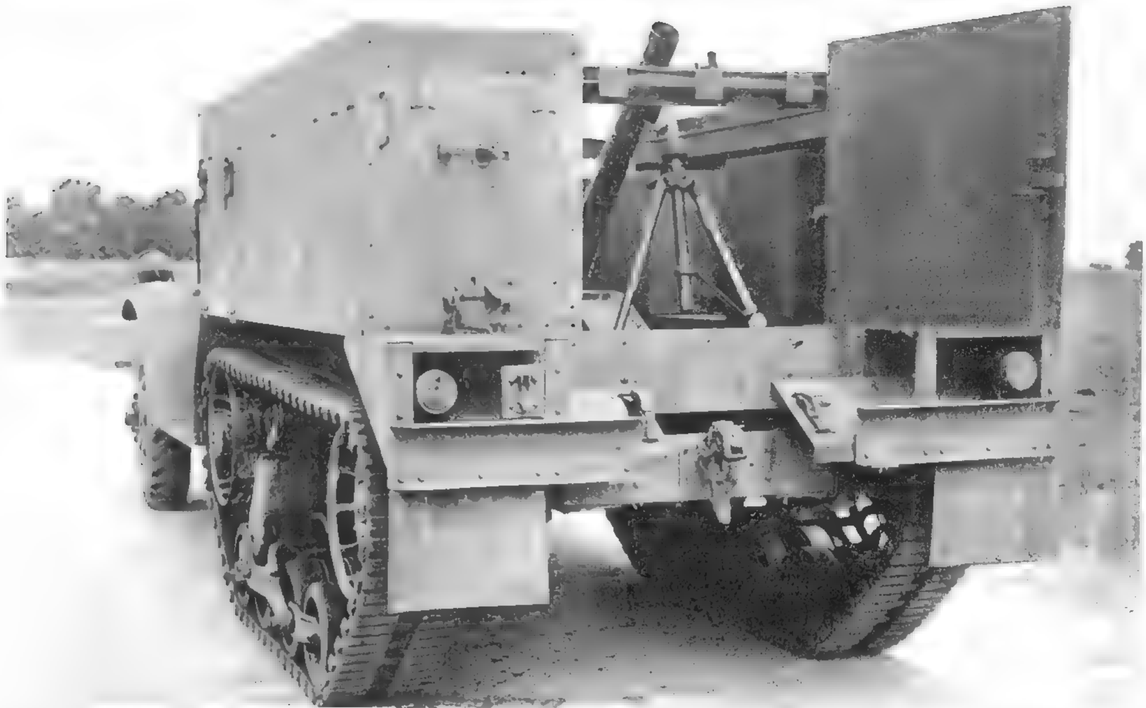
This photo shows why so many M4 crews chose not to dismount the 81mm mortar before firing. Notice how the skate rail crosses the rear door opening, making for a very small passage. The M4's lineage to the M2 is evident in this photo. Notice the rear "porch" characteristic of M2-based vehicles. (U.S. Army photo)
